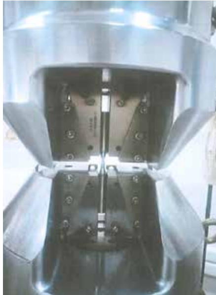
Figure 4: Test Configuration and Fatigue Limit Test Specimen [1]
