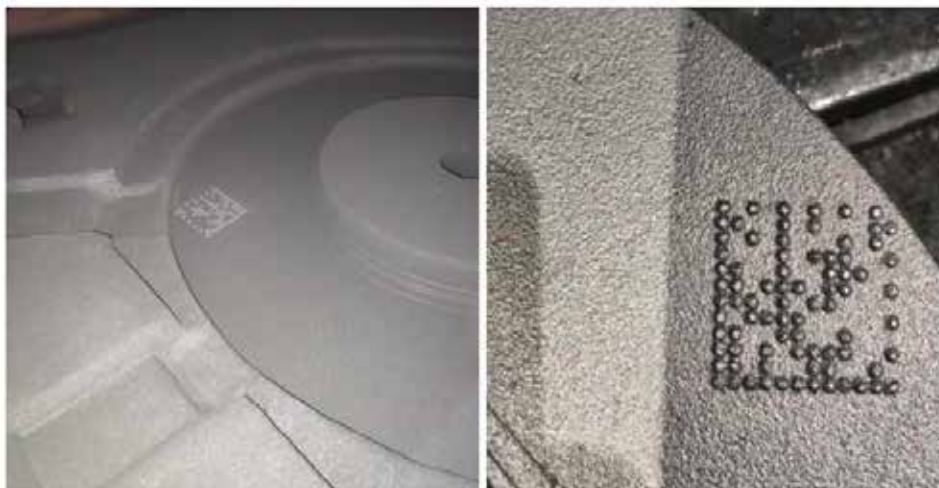
Figure 1 & 2: Unreadable, Low Contrast Data Matrix on Sand Mold and on Casted Part
