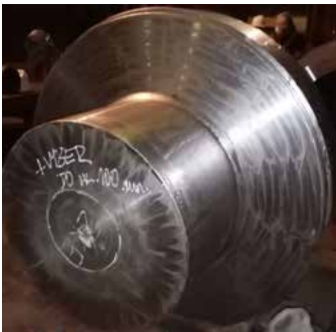
Fig 13a: Porosity in bottom hub
