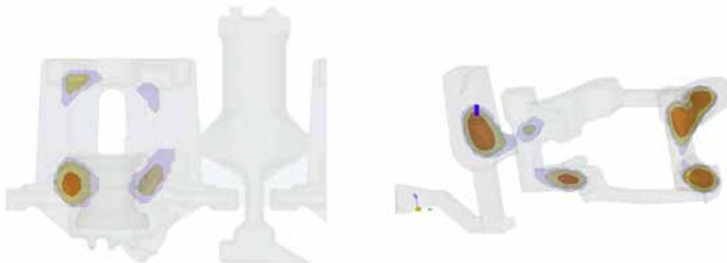
Figure 3: Cross section of a caliper and a holder in DI showing the different feeding isolated areas. Courtesy of Kasandra® software.
