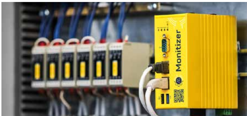
Figure 2: MAT Group's EURAC Poole, UK facility has connected Monitizer | DISCOVER to more and more equipment over the last six years to create a real-time, data-based view of its entire process.
