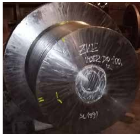
Fig 13b: Porosity under the riser
