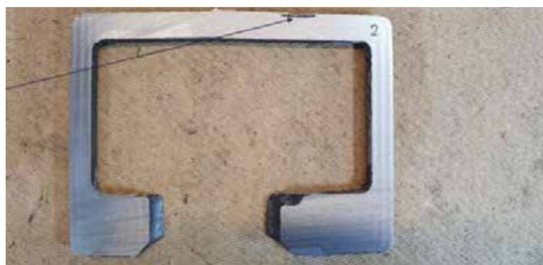
Figure 12 : Small gas porosity inclusion arrowed in casting section.
