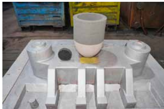
Figure 6: View of the feeding system on pattern
