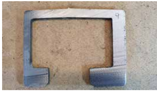
Figure 13 : Example of defect-free casting section.
