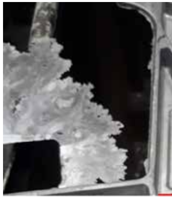
Figure 6: Flash formation due to exceeding mold closing force.
