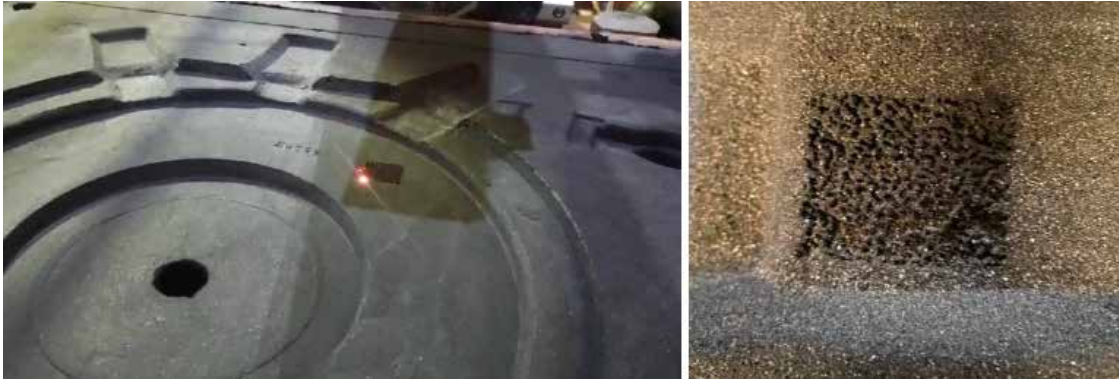
Figure 7 & 8: CDOT code second trial with 60W fiber laser with 110mm lens
