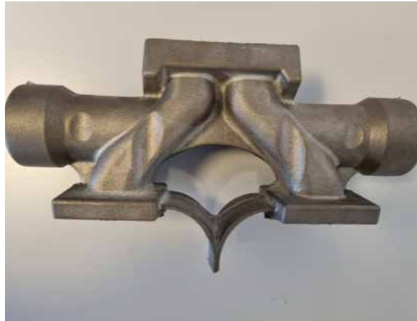
Figure 1 : A steel manifold produced in green sand.
