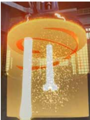
Fig 3a: Very fine Ar bubbles helically dispersed
