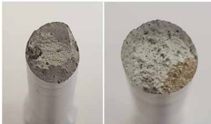
Figure 9: Fracture Surfaces of Specimen 3 and Specimen 6
