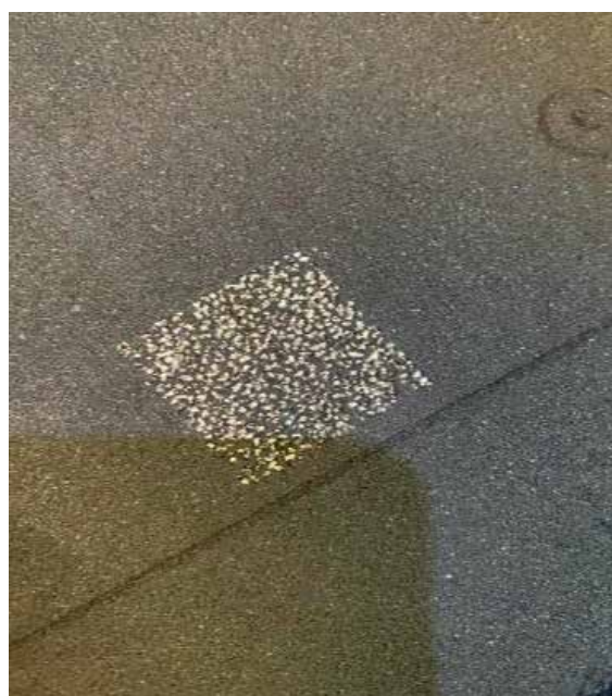
Figure 6: CDOT code first trial with 50W fiber laser with 300mm lens
