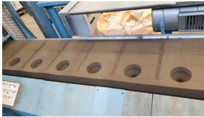
Figure 10 : Mould string ready for pouring.
